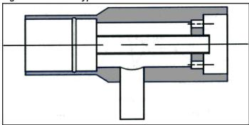
Figure 4: Hot Gas Bypass Kit (Installed)
