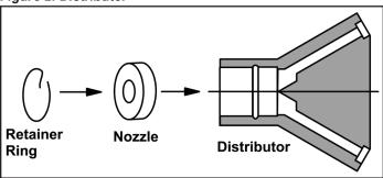
Figure 3: Hot Gas Bypass Kit
